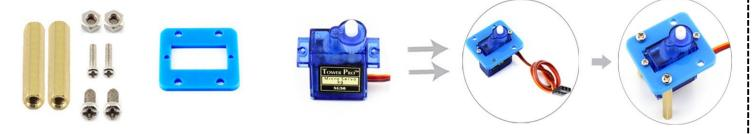
Fix the two-way rocker arm to the Pinboard with (E), and then install the Pinboard to the SG90 steering gear and use the screw (1.) to fix it. Finally, insert the ultrasonic sensor to the Pinboard.
