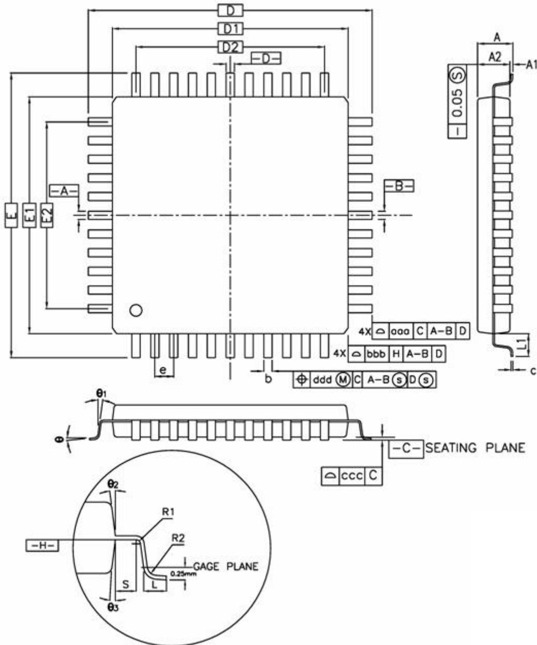
ⓘ Above diagram shows PIN dimension. All 80 pins are not displayed.
