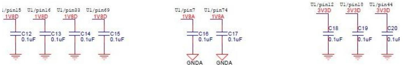
Place C12, C13, C14, C15, C16, C17, C18, C19, C20 as close to each power pin as possible.
