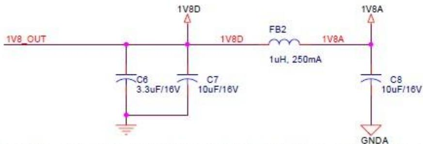
Place C6, C7, FB2 close to 1V8OUT and place C8 close to 1V8A
