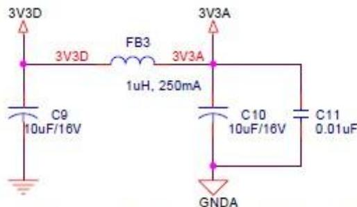
Place C9, FB3 close to 3V3D and place C10, C11 close to 3V3A
